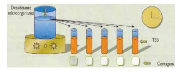
**FIGURE 2 -** Representation of decimal reduction time method (D value).
