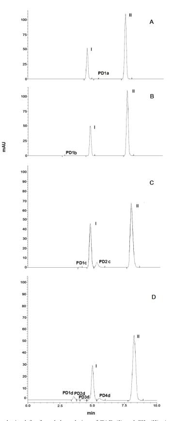
**FIGURE 3** - Chromatograms obtained for forced degradation of TAD (I) and SIL (II). A: acidic degradation; B: alkaline degradation; C: oxidative degradation; D: photolytic degradation; PD: likely degradation products.
