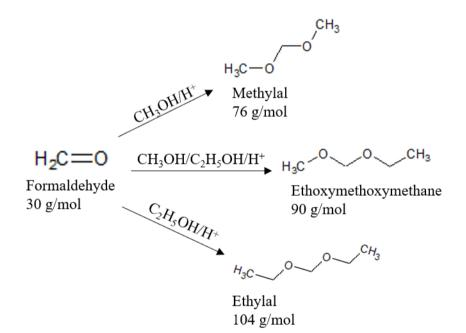
**FIGURE 1** - Derivatization of formaldehyde by acid catalytic reaction using methanol, ethanol and methanol/ethanol, showing the formation of the acetals methylal, ethoxymethoxymethane and ethylal.
