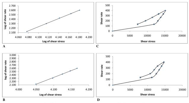
FIGURE 1 - Log shear stress vs. log shear rate plot of DSP<sub>5</sub> (A) and BSP<sub>5</sub> (B) Shear rate vs. shear stress plot of DSP<sub>5</sub> (C) and BSP<sub>5</sub> (D)
