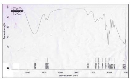
**FIGURE 4** - FTIR Spectra of the Dexamethasone sodium phosphate alone (A) and with excipients and polymers (B) in the optimized formulation DSP<sub>5</sub>
