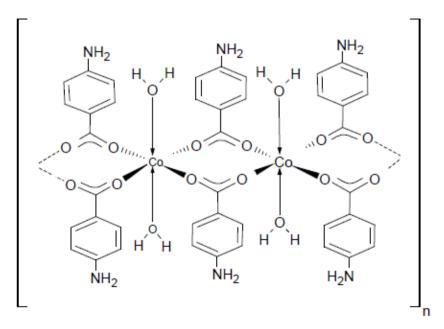
**FIGURE 4** – Structural representation of *catena*-poly-{[trans(diaqua-kO)cobalt(II)]-bis(*m*-*p*-aminobenzoato- $k^2O,O'$ )}.
