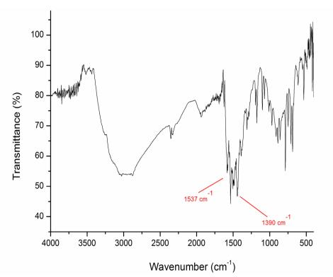
**FIGURE 5** – FT-IR spectrum of *catena*-poly-{[trans(diaqua-kO)cobalt(II)]-bis(*m*-*p*-(benzylideneamino)benzoato- $k^2O, O'$ )}.
