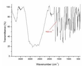
**FIGURE 1** – FT-IR spectrum of 4-(benzylideneamino)benzoic Acid.
