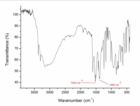
**FIGURE 3** – FT-IR spectrum of *catena*-poly-{[trans(diaqua-kO)cobalt(II)]-bis(*m*-*p*-aminobenzoato- $k^2O, O'$ )}.
