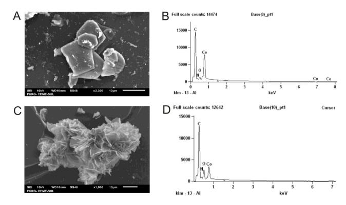
**FIGURE 8** – SEM-EDS results obtained for compound 5 (A)/(B) and for compound 4 (C/D).
