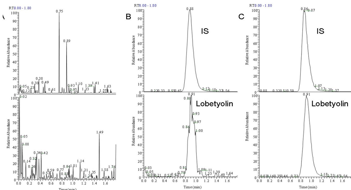
**FIGURE 2** - Representative MRM chromatograms (A) blank rat plasma; (B) blank rat plasma spiked with lobetyolin and IS; (C) real plasma sample 1 h after oral dose of 10 mg/kg.
