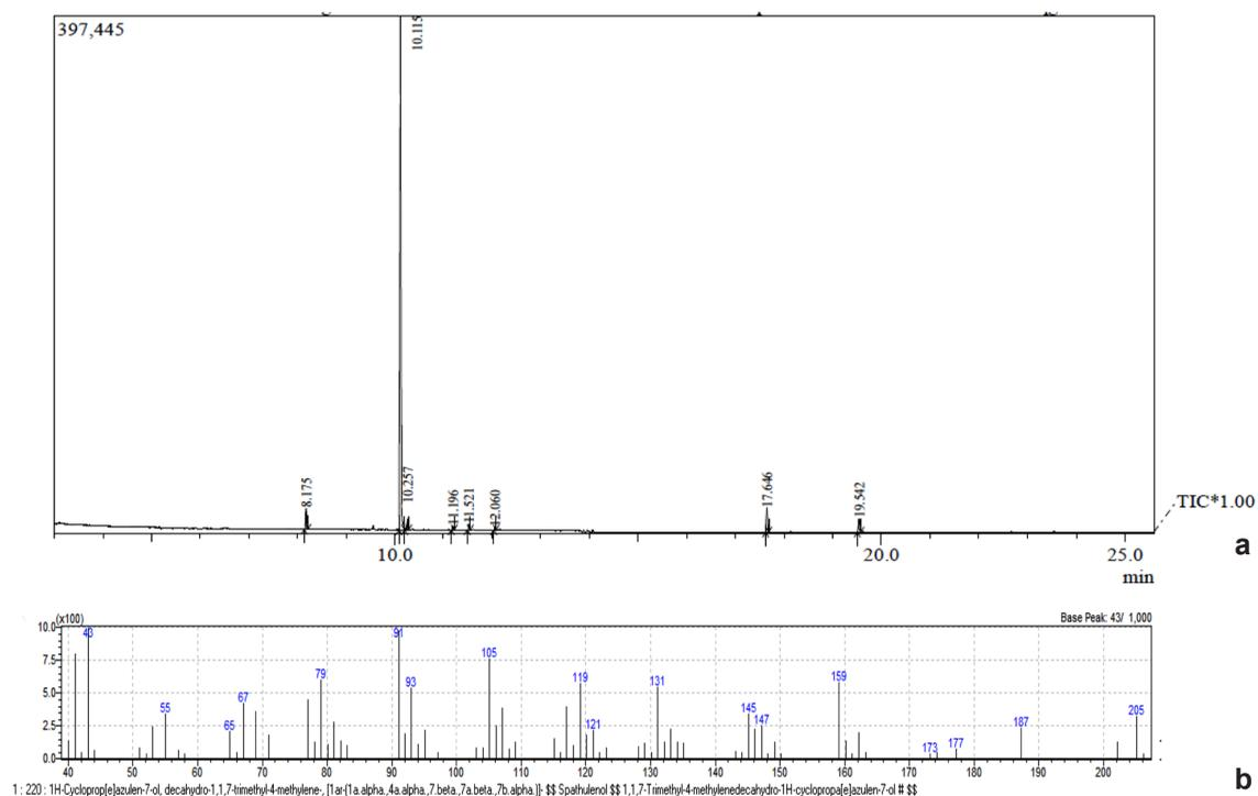
**Figure 1** – a. Chromatogram of the SF5 obtained by gas chromatography coupled with mass spectrometer (GC-MS). b. Mass spectrum of the major peak at t<sub>R</sub> 10.115 min, spathulenol.
