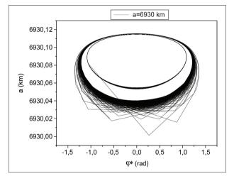
Figure 2. Semi-axis versus critical angle: e=0.019, i=87° e \u03c6\*=0.
