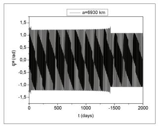
Figure 5. Variation of critical angle in the time: e=0.019, i=87° e  $\phi$ \*=0.
