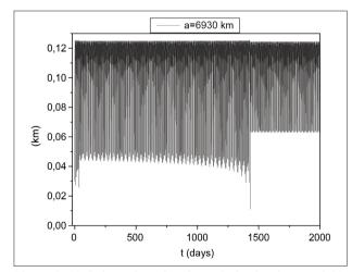
Figure 3. Variation of semi-major axis in the time: e=0.01,  $i=4^{\circ}, \phi^*=0^{\circ}$ .
