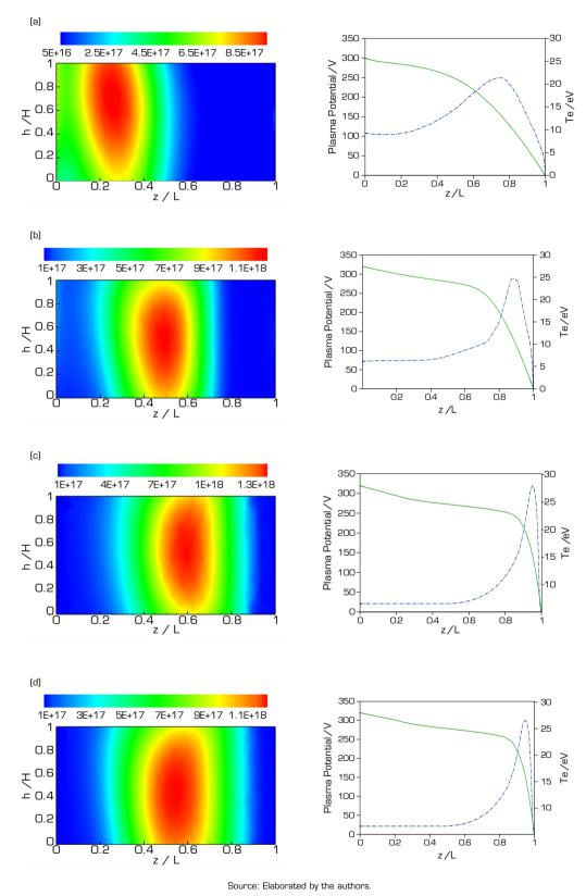
**Figure 5.** Distribution of the electron density in the discharge channel ( $m^{-3}$ ) and the potential and the electron temperature along the center line of the channel when Br-max is 110 Gs (a), 170 Gs (b), 200 Gs (c), 220 Gs (d).
