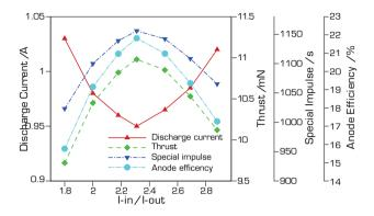
Source: Elaborated by the authors. Figure 14. Performance of the thruster with different  $\frac{I_{ln}}{I_{out}}$ .
