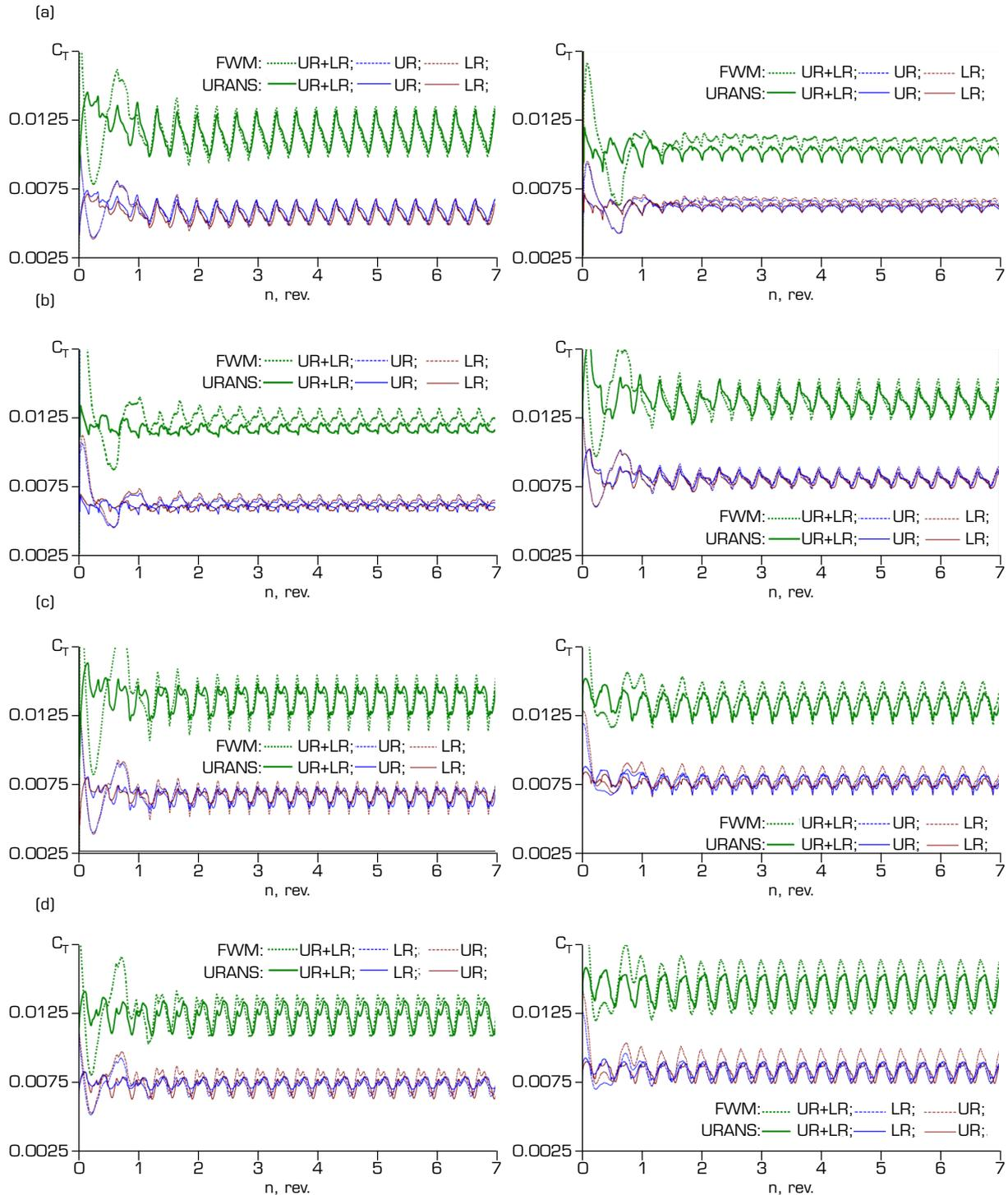
**Figure 14.** Calculated dependences of instantaneous thrust and torque coefficients vs. number of rotor revolutions based on the FWM and the URANS. (a)  $V = 30 \text{ m}\cdot\text{s}^{-1}$ ;  $\alpha_R = -4.7^\circ$ ; (b)  $V = 40 \text{ m}\cdot\text{s}^{-1}$ ;  $\alpha_R = -7.3^\circ$ ; (c)  $V = 50 \text{ m}\cdot\text{s}^{-1}$ ;  $\alpha_R = -10.4^\circ$ ; (d)  $V = 60 \text{ m}\cdot\text{s}^{-1}$ ;  $\alpha_R = -14.4^\circ$ .
