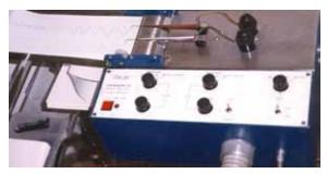
FIGURE 5 - Device used to perform the active anterior rhinomanometry exam. Rhinomanometer RM - 302 from Berger<sup>TM</sup>.
