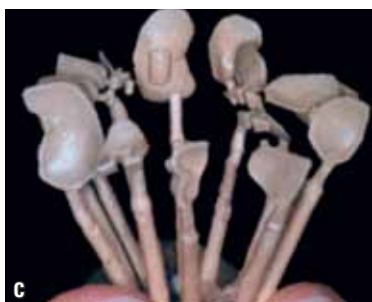
FIGURE 12 - Casting process of brackets.
