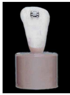
FIGURE 5 - Specimen with bracket bonded to buccal surface.
