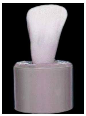
FIGURE 2 - Bovine tooth inserted in PVC tube.
