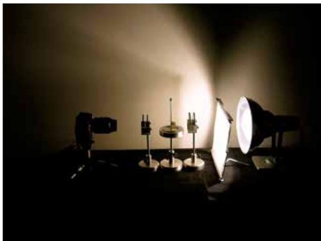
Figure 1 - Circular polariscope.
