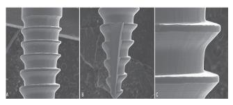
Figure 3 - Photomicrographs of the mini-implants studied. A) Area next to the transmucosal profile where mechanical fracture resistance test was performed (x50); B) Area next to the tip where mechanical fracture resistance test was performed (x50); C) Image of mini-implant body (x150). Smooth surface without defects, and tip with a cutting area.
