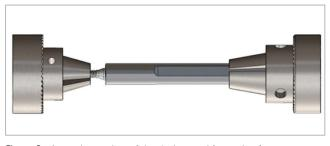
Figure 2 - Approximate view of the device used for testing fracture torque, showing one MI attached to one grip and the insertion-removal key attached to other.
