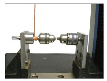
Figure 1 - Device used for mini-implant torsional tests
