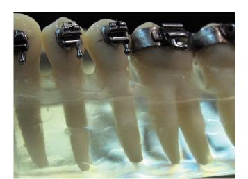
Figure 1 - Photoelastic model without residual tension.
