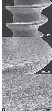
Figure 1 - Electromicrographs of smooth (A) and rough (B) mini-implant surfaces.
