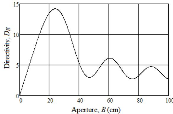
Fig. 3. Directivity curve computed with respect to the aperture  $B$  with  $R_2=23.65$  cm for an operating frequency of 2.5 GHz using a WR430 waveguide.
