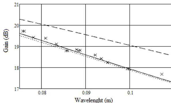
Fig. 2. Gain curves obtained for a WR284 waveguide with  $A = 32.41$  cm,  $B = 24$  cm,  $l_E = 42.15$  cm and  $l_H = 47.45$  cm. — analysis using exact phase errors, .....analysis using quadratic phase errors, - - - analysis using quadratic phase error in  $H$ -plane and Jull's formula in the  $E$ -plane [7], xxx measured values [4],[8].
