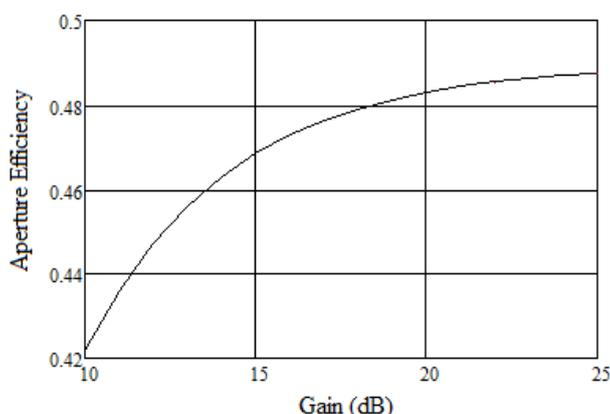
Fig. 4. Variation of the aperture efficiency obtained from the optimum design with a WR430 waveguide and a frequency of 2.5 GHz.
