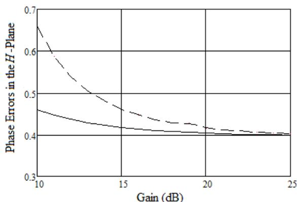
Fig. 5 Variation of the phase errors in the  $H$ -plane with respect to the desired gain obtained from the optimum design with a WR430 waveguide and a frequency of 2.5 GHz. — Exact phase error, - - - Quadratic phase error.
