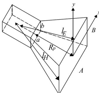
Fig. 1. Geometry of a pyramidal horn antenna.
