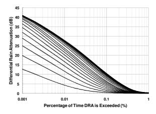
Fig. 6. Cumulative distribution functions of the differential rain attenuation presented from left to right for angles varying between 5° and 50° with 5° increments and between 50° and 180° with 10° increments, assuming vertically-polarized 15-GHz links located in the São Paulo region ( $d_o = 6.80$  km and  $\beta = 0.52$ ) with fixed path lengths  $D_1 = D_2 = 10$  km.
