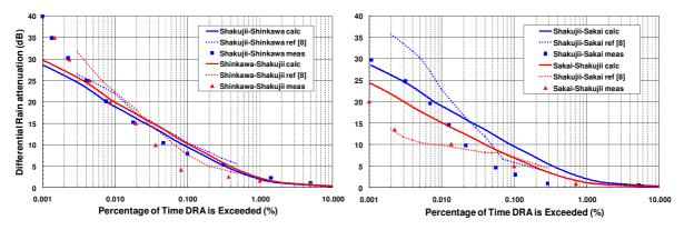
Fig. 4. Calculated (continuous and dashed curves) and measured (filled symbols) cumulative distribution functions for the differential rain attenuation between the converging ECL links described in Section III (adapted from reference [4]).
