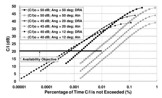
Fig. 8. Cumulative distribution functions of the ratio C/I for the conservative (dashed lines with hollow symbols) and realistic (continuous lines with filled symbols) procedures, and three values of the ratio  $(C/I)_0$  (or, equivalently, three angle between the converging links), as well as the availability objective adopted in link design
