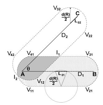
Fig. 1. Converging links AB and AC with respective path lengths  $D_1$  and  $D_2$  making the angle  $\theta$  at the common terminal, associated geometric loci  $V_{11}V_{21}I_1V_{31}V_{41}I_2$  and  $V_{12}I_1V_{22}V_{32}V_{42}I_2$  corresponding to attenuations  $A_{o1}$  and  $A_{o2}$ , respectively, and to a cylindrical cell of rainfall rate R, as well as the intersection  $V_{12}I_1V_{41}I_2$  between the two geometric loci.
