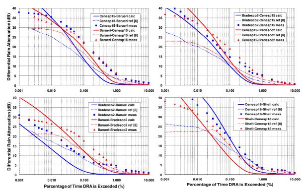
Fig. 5. Calculated (continuous and dashed curves) and measured (filled symbols) cumulative distribution functions for the differential rain attenuation between the converging RIS links described in Section III.
