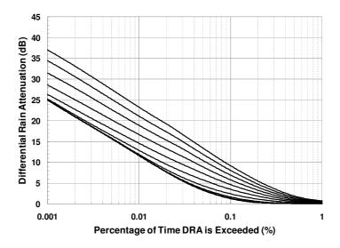
Fig. 7. Cumulative distribution functions of the differential rain attenuation presented from right to left for increasing values of the path length  $D_2$  (from 3 km to 15 km in 1-km increments), assuming vertically-polarized 15-GHz links located in the São Paulo region( $d_o = 6.80$  km and  $\beta = 0.52$ ) with fixed path length  $D_1 = 10$  km and angle  $\theta = 15^\circ$ .
