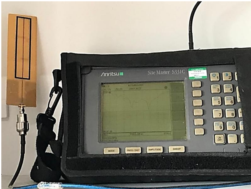
Fig. 4. The return loss measurement setup.
