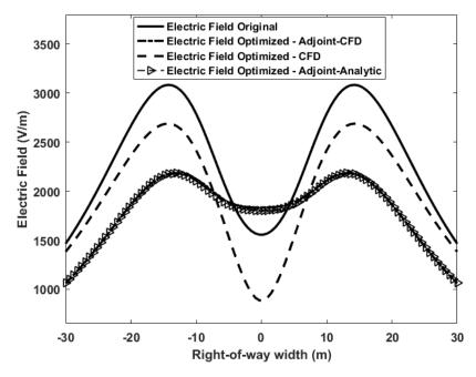
Fig. 2. Electric field profile at the ground level - original and optimized.
