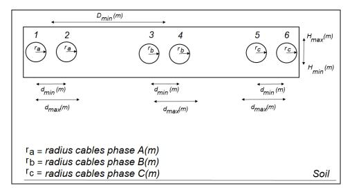
Fig. 1. Geometric constraints adopted during optimization process:  $D_{min}$  is the minimum distance between conductors of different phases;  $d_{min}, d_{max}$  are the respective: minimum and maximum distance between conductors of the same bundle;  $H_{min}, H_{max}$  are the respective: minimum and the maximum height of each cable.
