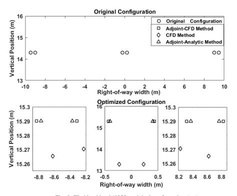
Fig. 3. TL 02 cables 345kV - original configuration (  $\circ$  ), optimized configuration: adjoint-CFD method (  $\Box$  ), adjoint-analytic method (  $\triangle$  ), CFD method (  $\diamond$  ).
