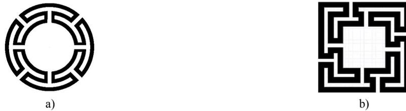
Fig. 4. Polarization independent matryoshka geometry: a) Matryoshka circular ring, b) Matryoshka square ring
