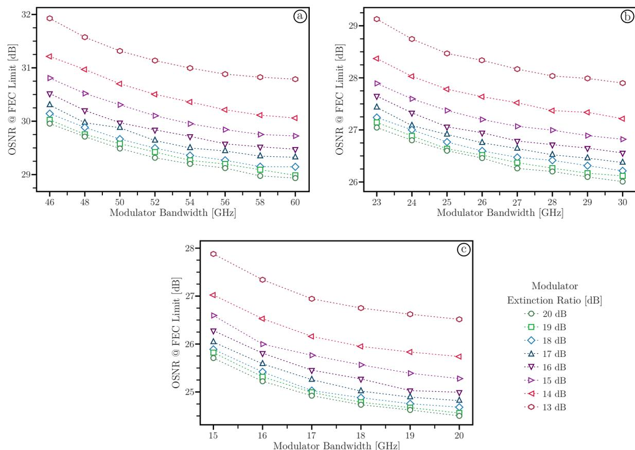
Fig. 2. OSNR required at the FEC limit as a function of modulator bandwidth ( $B_{mod}$ ) and extinction ratio ( $ER_{mod}$ ) in back-to-back transmission of a 1-Tb/s superchannel employing (a) 1, (b) 2, or (c) 3 optical carriers. OSNR is the ratio of total signal power of an optical carrier to noise power in a reference bandwidth of 0.1 nm.
