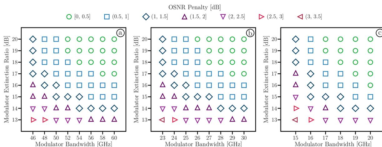
Fig. 3. OSNR penalty as a function of modulator bandwidth ( $B_{mod}$ ) and extinction ratio ( $ER_{mod}$ ) in back-to-back transmission of a 1-Tb/s superchannel employing (a) 1, (b) 2, or (c) 3 optical carriers.
