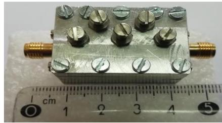
Fig. 13. Photo for the fabricated dual-band filter.
