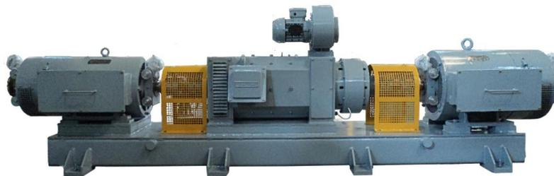
Fig. 6. Experimental test bench with a 10 kVA, 8-pole synchronous generator.
