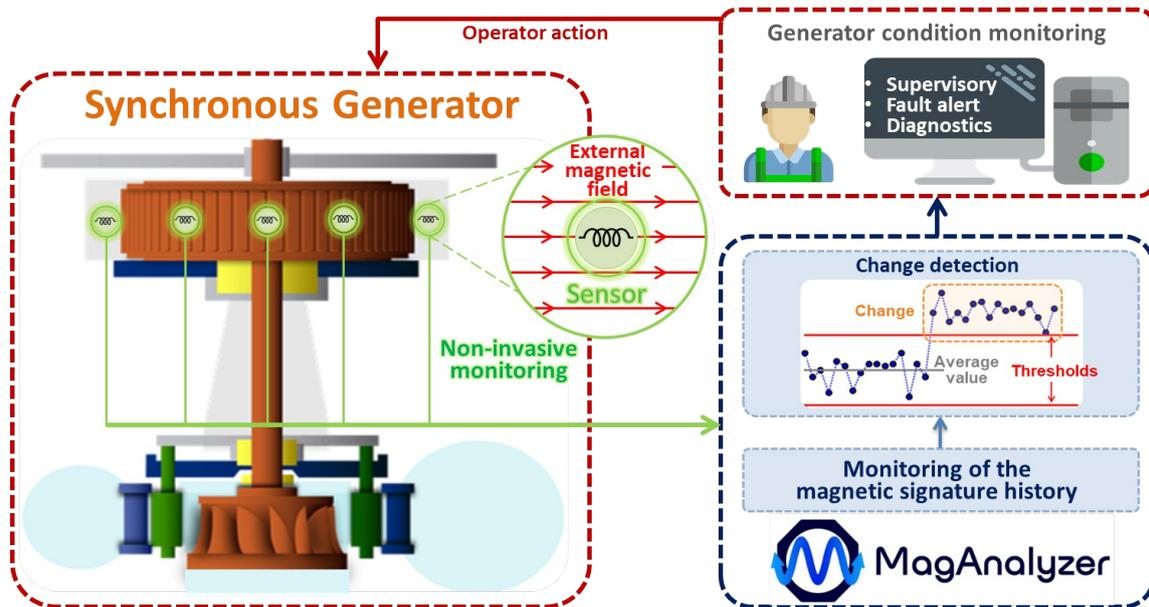
Fig. 1. Generic architecture of MagAnalyzer monitoring system.
