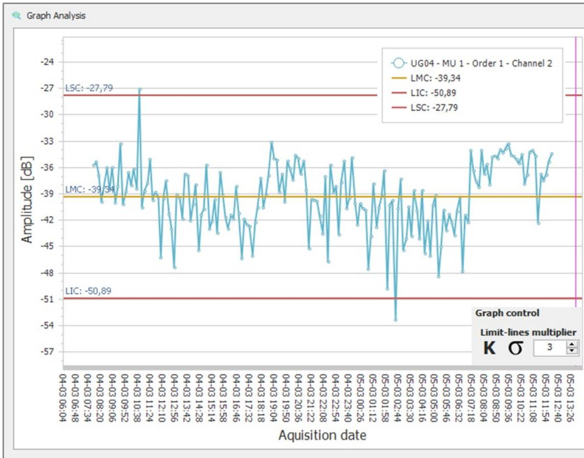
Fig. 13. SG magnetic signature viewing and analysis window in the monitoring software.
