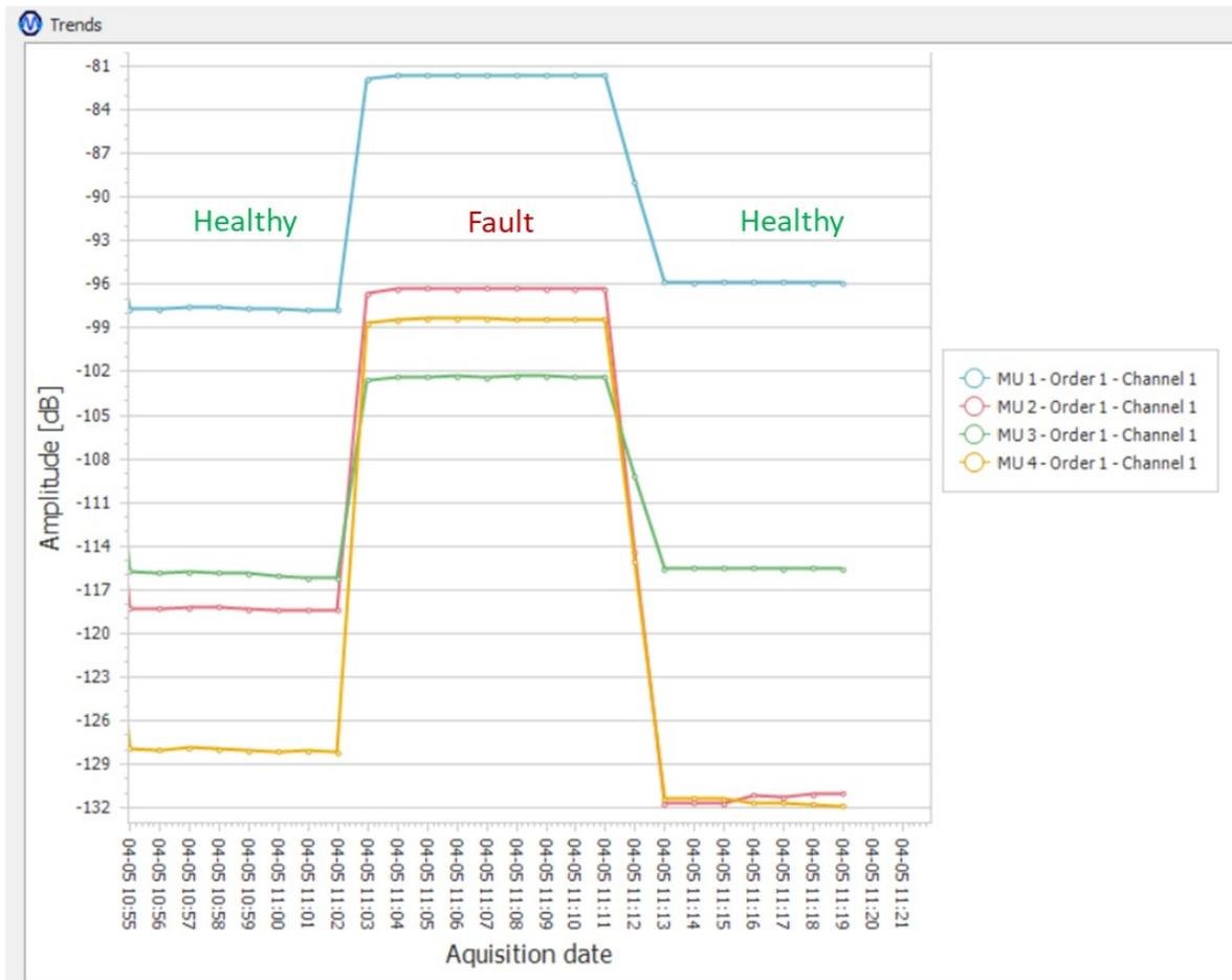
Fig. 20. Amplitudes history of the mechanical rotation frequency in 4 MUs face to the fault.
