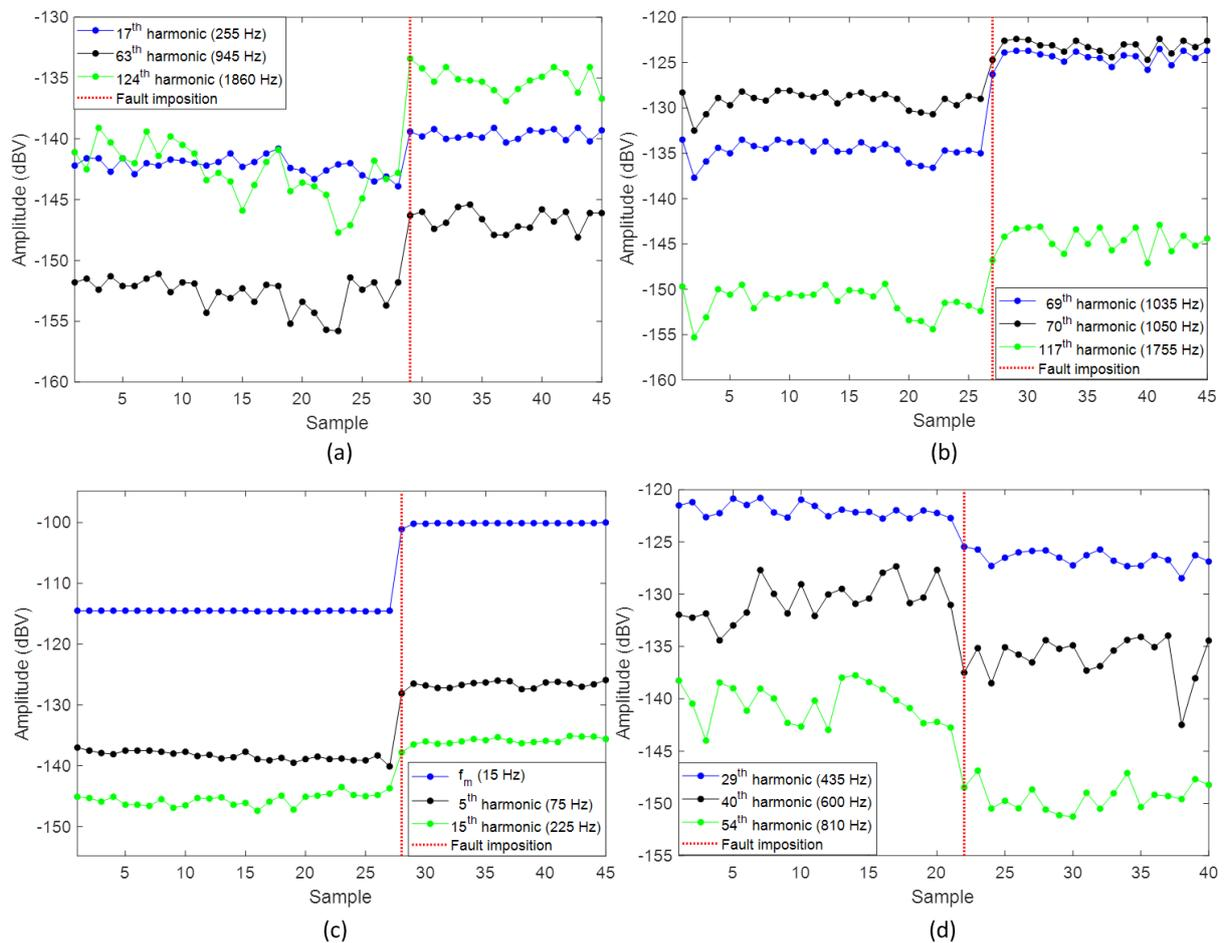
Fig. 7. Tests with controlled fault imposition on the experimental test bench: (a) removal of turns from one pole of the stator, (b) short-circuit between stator core sheets, (c) removal of turns from one pole of the rotor, (d) dynamic unbalance (mechanical vibration).
