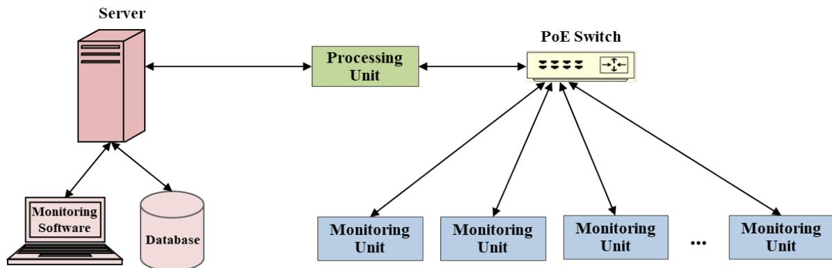
Fig. 9. MagAnalyzer system architecture.
