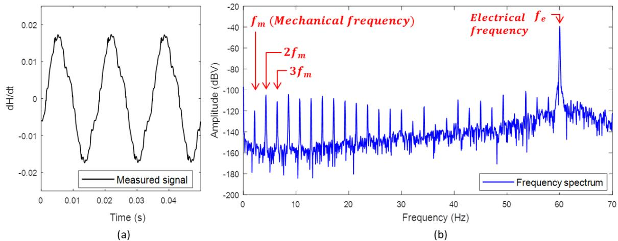
Fig. 16. (a) Waveform of the external magnetic field time derivative, (b) frequency spectrum of the signal.
