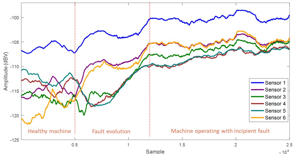
Fig. 8. Amplitude history of the 141<sup>st</sup> harmonic of the mechanical rotation frequency during the fault evolution.
