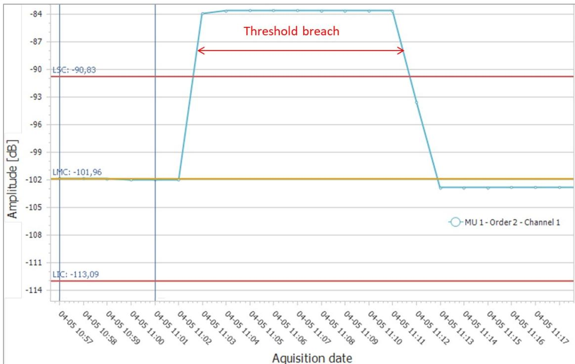
Fig. 21. Application of control charts for fault detection with the MagAnalyzer system monitoring software.
