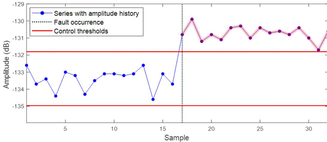
Fig. 5. Application of the control chart method in the detection of magnetic signature changes.
