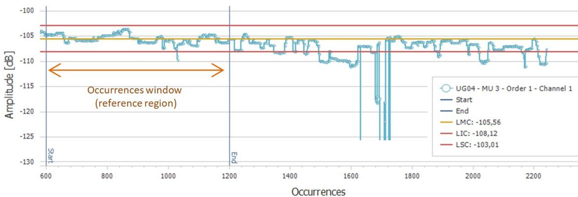
Fig. 19. Applying control charts for detecting trend changes.
