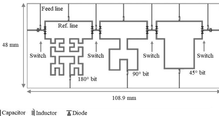
Fig. 4. Proposed fractal-based phase shifter.
