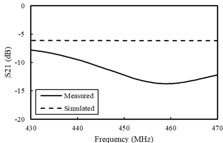
Fig. 7. Simulated and measured  $|S_{21}|$  for its 0 degrees phase shift.
