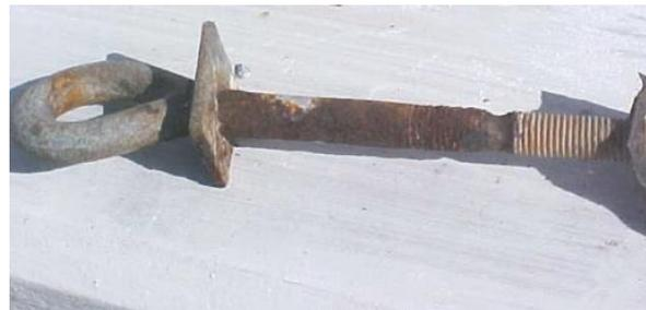
Fig. 2. Effect of corrosive process in eye bolts
