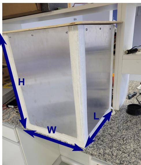
Fig. 6. Cavity under test, dimensions  $W=L= 46$  cm and  $H= 61$  cm.
