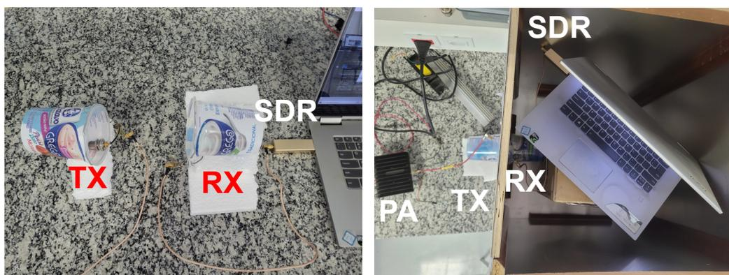
Fig. 9. (Left) both coils and the SDR and, (right) laptop, SDR and RX coil placement inside the cavity, top view.
