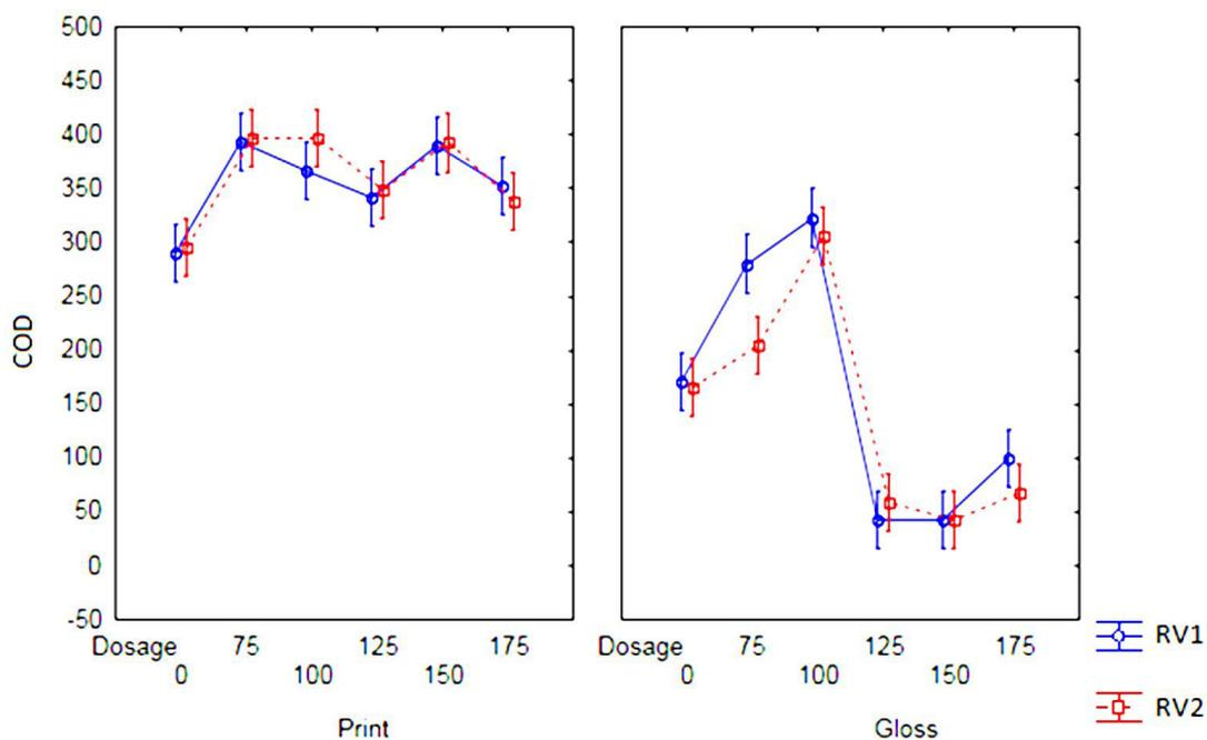
**Figure 3.** Interaction between: dosage x rise velocity x paper type for COD.
