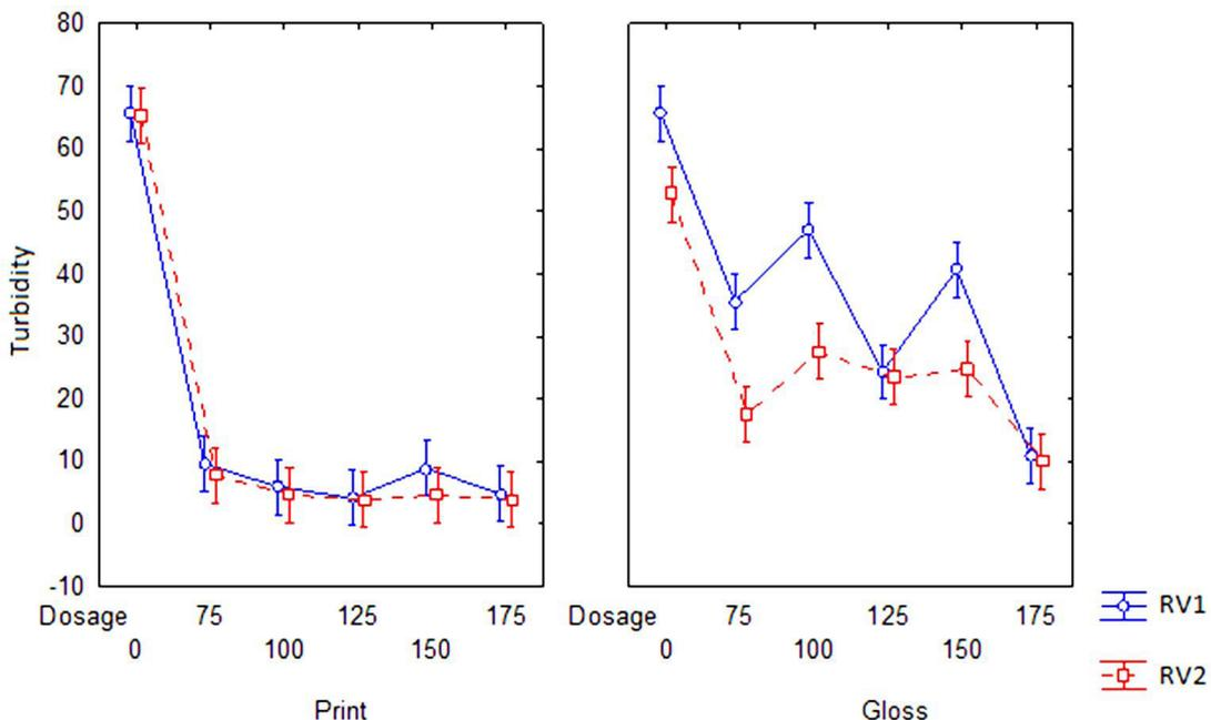
Figure 2. Interaction between: dosage x rise velocity x paper type for turbidity.
