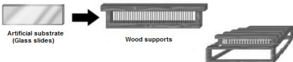
Figure 2. Artificial substrate used in the experiment (Adapted from Murakami, 2008).
