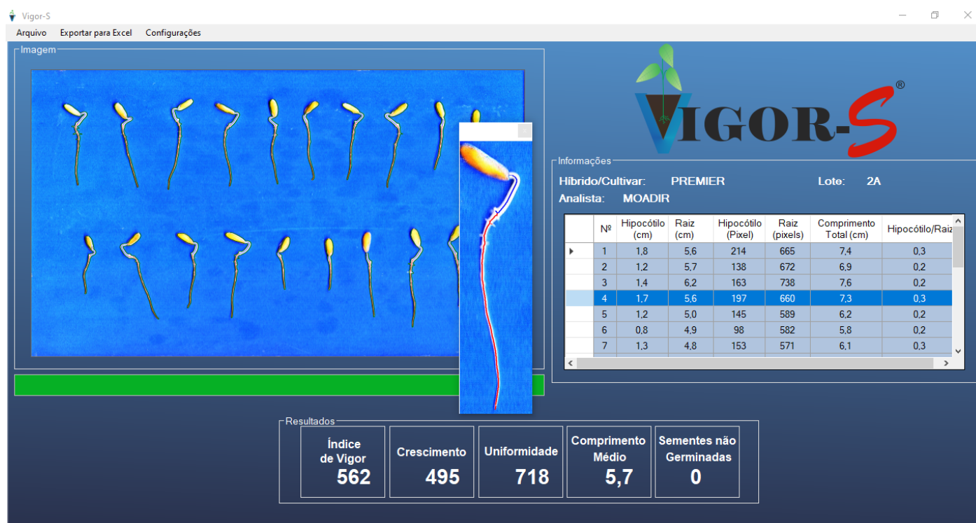
Figure 1. General aspects of the analysis of Cucumis melo L. seedlings by the software Vigor-S, highlighting the hypocotyl (blue color) and root (red color).
