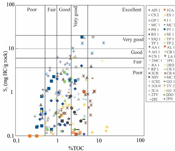
**Figure 8.** Hydrocarbon source potential ( $S_2$ ) versus total organic carbon (TOC) of the Irati Formation (Assistência Member) in wells with igneous intrusions or with intrusions close to the Irati Formation. Most samples are characterized by a low hydrocarbon source potential due to thermal depletion caused by intrusive rocks depletion according to Peters and Cassa (1994) classification.
