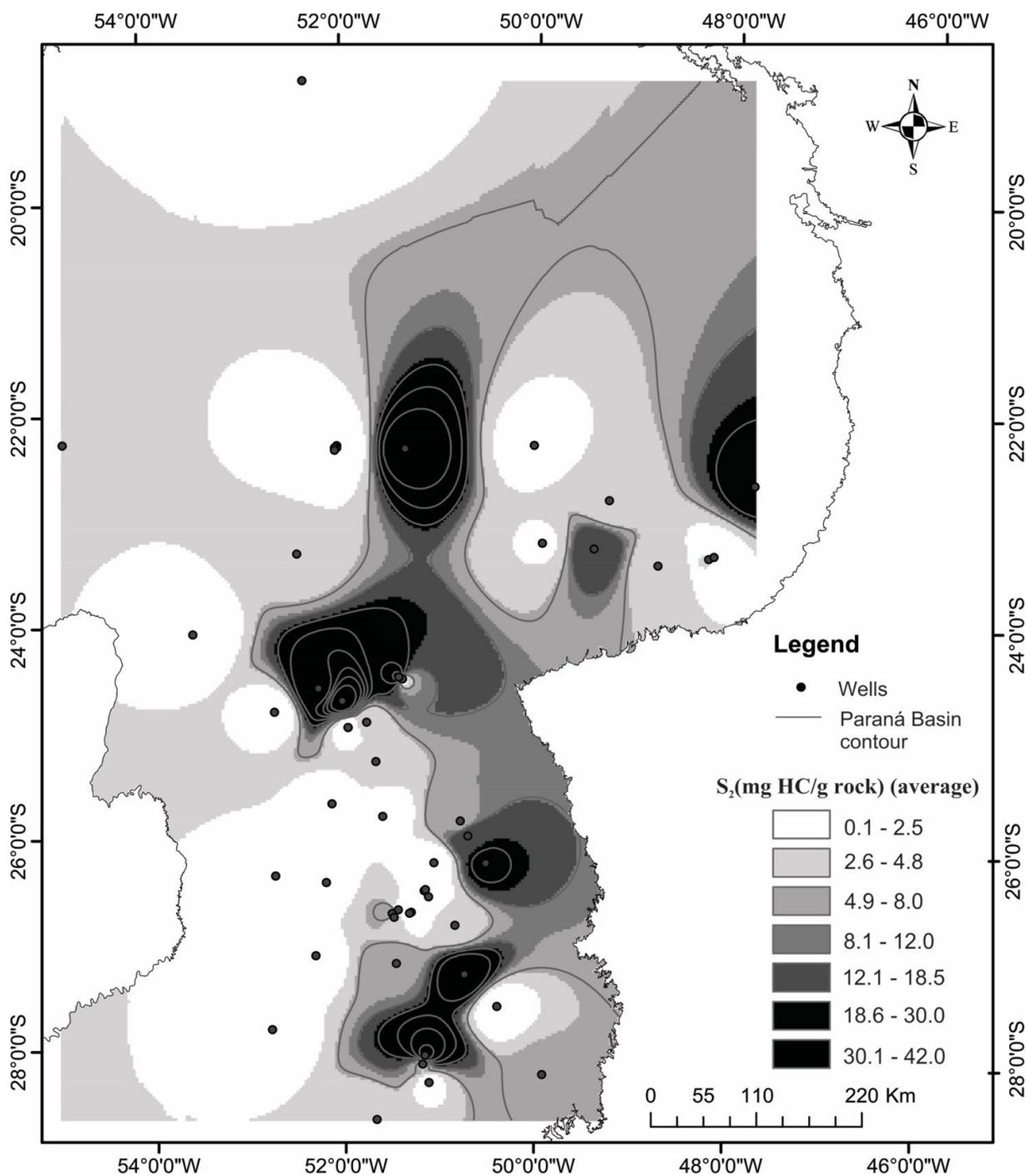
**Figure 5.** Residual average of source rock potential of the Irati Formation (Assistência Member) (S<sub>2</sub> — mg HC/g rock).
