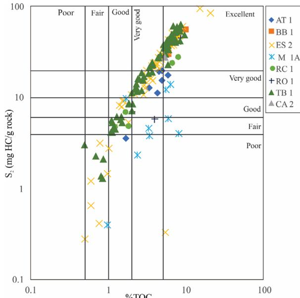
**Figure 7.** Hydrocarbon source potential ( $S_2$ ) versus total organic carbon (TOC) of the Irati Formation (Assistência Member) in wells without igneous intrusions. Most samples are characterized by a good to excellent hydrocarbon source potential according to Peters and Cassa (1994) classification.
