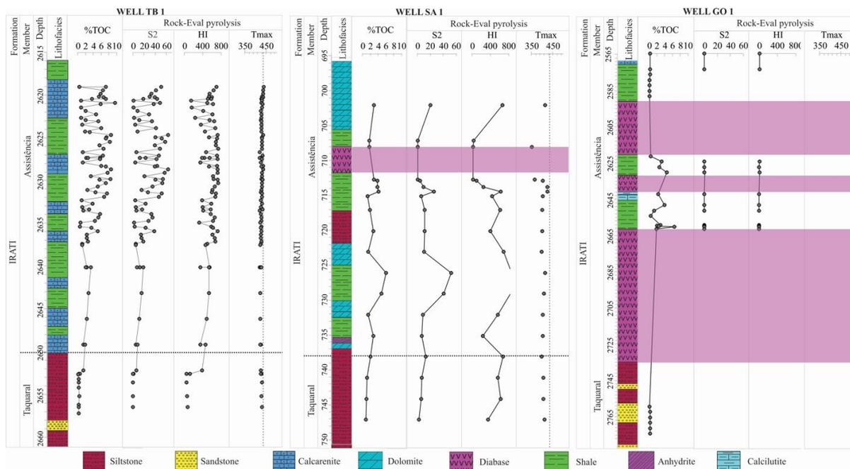
**Figure 12.** In-depth TOC, S<sub>2</sub>, HI, and T<sub>max</sub> logs of source rock samples and correlations in the wells studied. The Irati Formation comprises the Taquaral and Assistência Members, with the igneous intrusions highlighted.
