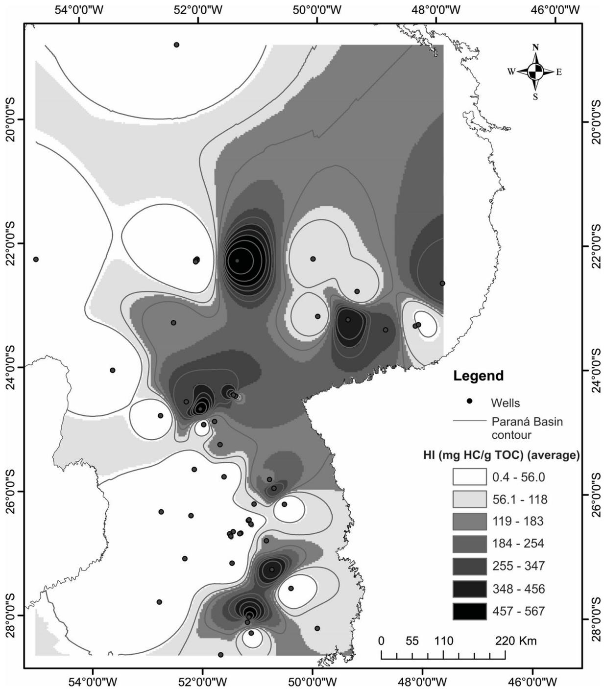
**Figure 6.** Residual average of the hydrogen index of the Irati Formation (Assistência Member) (HI — mg HC/g TOC).
