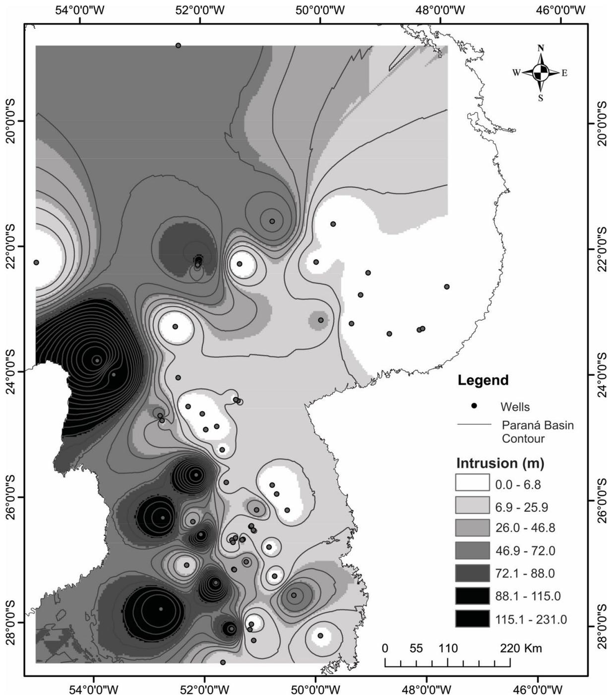
**Figure 4.** Map of the thickness of igneous intrusion in the Irati Formation, Paraná Basin. The higher the thickness, the higher the thermal stress range.
