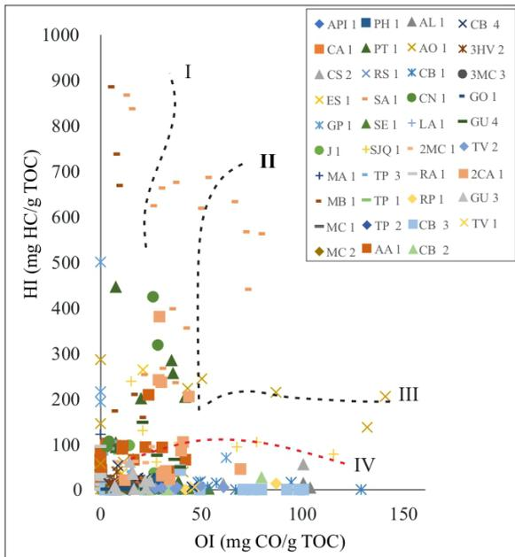
Source: modified from Euzébio *et al.* (2016). **Figure 11.** Van Krevelen diagram showing the distribution of the analyzed samples from the wells with diabase intrusions, highlighting the presence of type IV kerogen due to severe depletion of HI caused by thermal stress.
