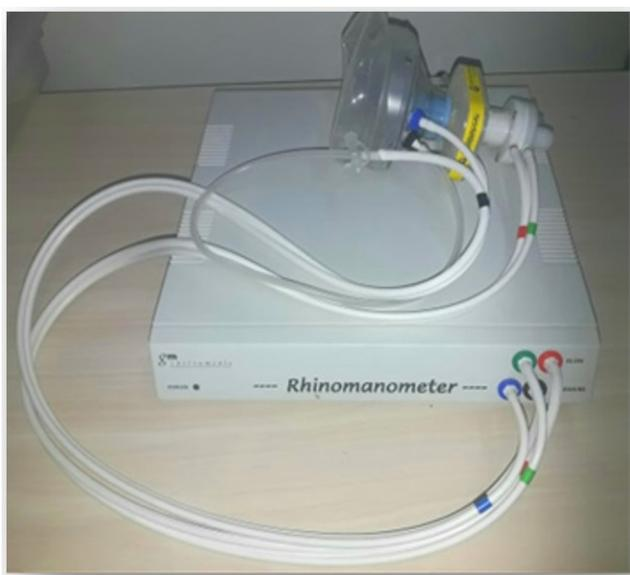
**Figure 1.** Rhinomanometer NR6. Adapted from GM Instruments
