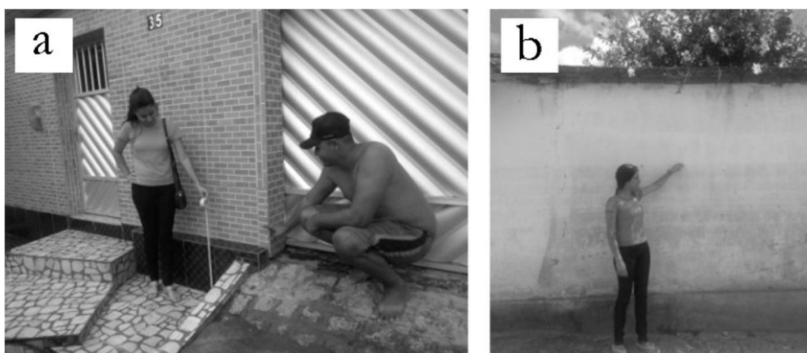
Figure 5. Data collection in the field. (a) Flood height measurement; b) Flood marks collection.
