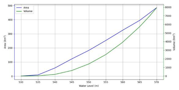
Figure 5. Level x Area x Volume curve of the Hydro Power Plant Jurumirim reservoir.
