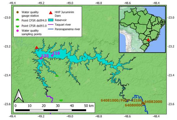
Figure 6. Positioning of the reservoir, water quality monitoring stations and monitoring points inside the reservoir used for calibration.
