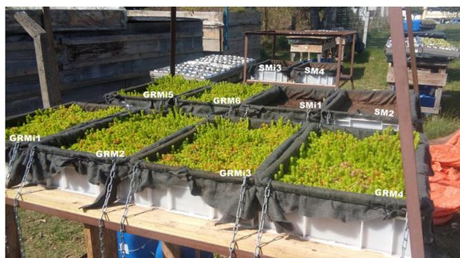
**Figure 1.** Experimental set up. Green Roofs Modules (GRM). Soil Modules (SM).
