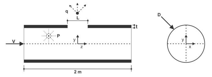
Figure 1. Definition sketch for a typical pipe of a water distribution system along the line x = 0, y = D/2, z = 0.
