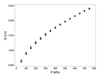
**Figure 2.** Comparison of the simulated leakage flow rate as a function of the pressure with the experiment of Coetzer (2006). Experimental: circles; computational: squares. V = 1 m/s, D = 110 mm, leak diameter = 1 mm. The maximum difference between numerical and experimental results was 7.1%. Coarse grid, with 36,633 elements (solid black lines); medium grid, with 49,212 elements (solid gray lines); fine grid, with 223,148 elements (dashed gray lines).
