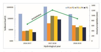
**Figure 4.** Total sediment transport at the hydrosedimentometric stations and accumulated annual precipitation. Pandeiros River – MG. Source: modified from Bandeira et al. (2020b).
