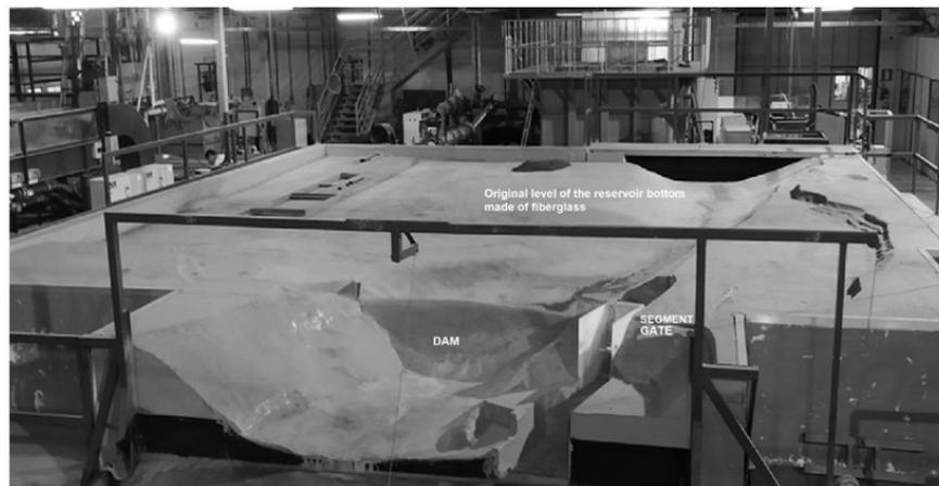
Figure 12. Top view of the reduced Model 02 of SHPP Salto Paraopeba (Fundação Cristiano Ottoni, 2013) and physical Model 02, where the fiberglass is already installed.
