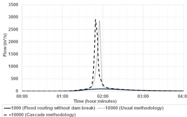
Figure 15. Hydrographs for comparing methodologies with minimum breach formation time according to Von Thun & Gillette (1990) and MacDonald & Langridge-Monopolis (1984) and cascade methodology.
