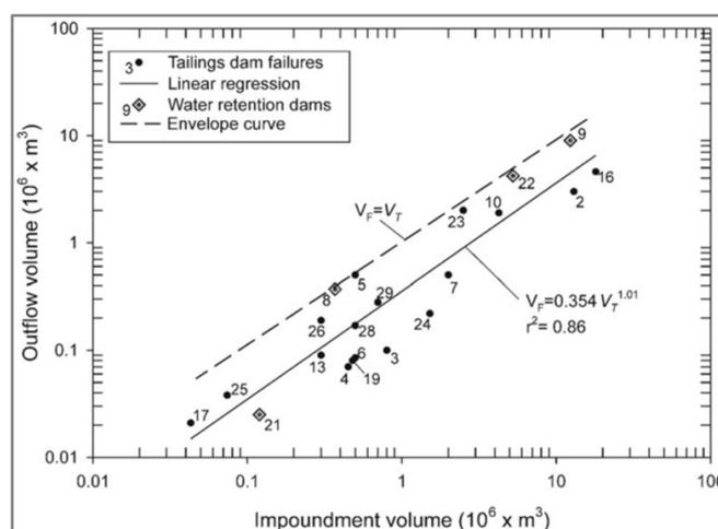
Figure 4. Impoundment volume and outflow volume [adapted from Rico et al. (2008)].
