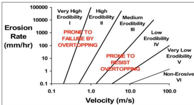
Figure 9. Guidelines for overtopping resistance [adapted from Briaud et al. (2008)].
