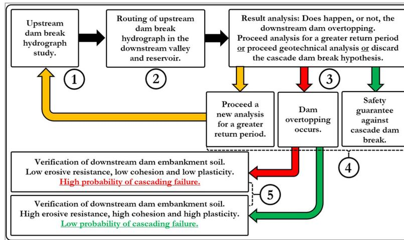
Figure 8. Flowchart for evaluating the occurrence of cascade rupture.
