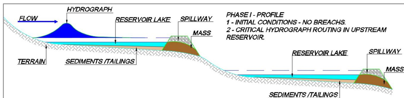
Figure 3. Preview of cascade dam break process – Phase I.
