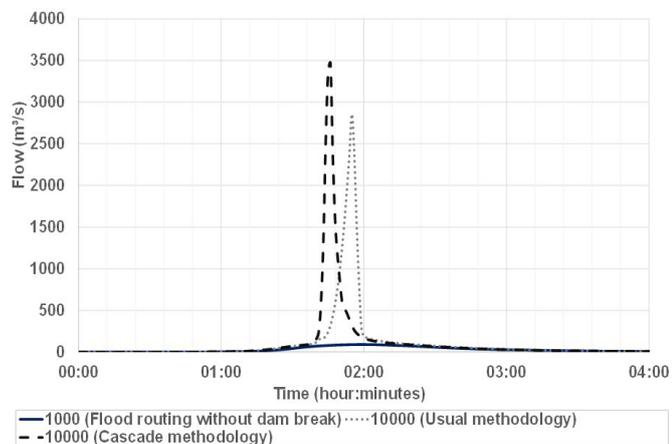
Figure 14. Hydrographs comparison of methodologies with minimum breach formation time according to Froehlich (2008) and cascade methodology.
