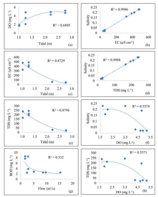
**Figure 5.** Regression analysis with data from Igarapé Tucunduba, data collected April 9, 2013: a) DO and tidal, b) salinity and EC, c) EC and tidal, d) salinity and TDS, e) TDS and tidal, f) salinity and DO, g) BOD and flow, h) TDS and DO.
