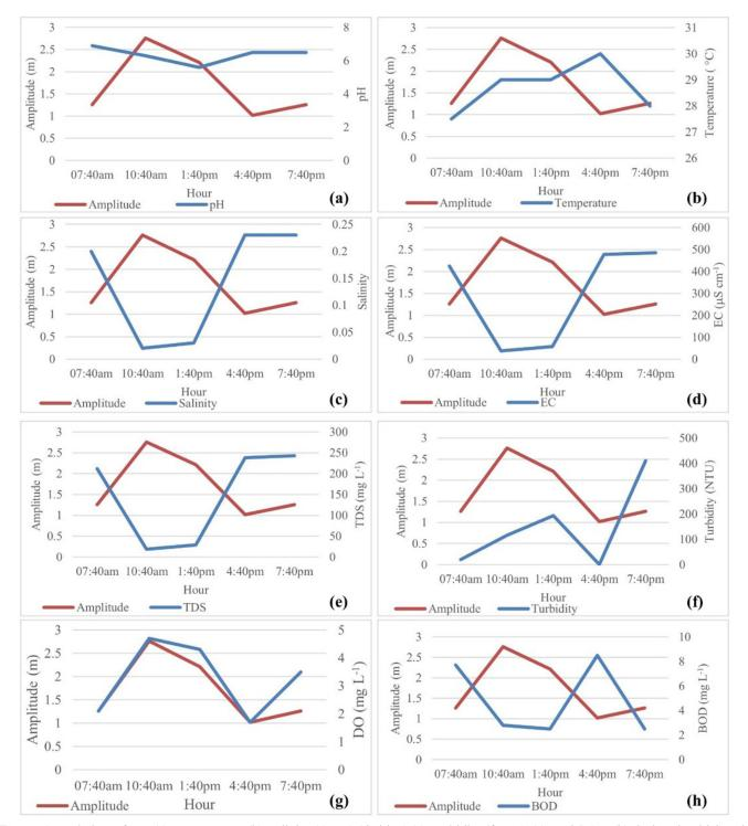
Figure 3. Variation of pH (a), temperature (b), salinity (c), EC (d), TDS (e), turbidity (f), DO (g), and BOD (h) during the tidal cycle in the Tucunduba Igarapé, data collected April 9, 2013.
