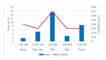
**Figure 4.** Distribution of the BOD load, with the maximum value recorded at the moment of greatest entry of the waters of the Igarapé Tucunduba, data collected April 9, 2013.
