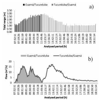
**Figure 2.** Dynamics of tide (a) and waste flow (b) of Tucunduba igarapé, data collected April 9, 2013.
