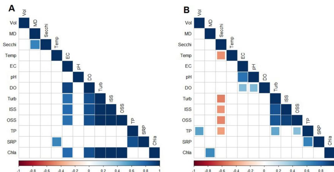
**Figure 4.** Pearson's correlation of the thirteen variables of the two periods in Cruzeta Reservoir (A) and Dourado Reservoir (B). Water Volume (Vol); Maximum Depth (MD); Secchi transparency (Secchi); Water temperature (T. water); Electrical Conductivity (EC); pH; Dissolved Oxygen (DO); Turbidity (Turb); Inorganic Suspended Solids (ISS); Organic Suspended Solids (OSS); Total Phosphorus (TP); Soluble Reactive Phosphorus (SRP) and Chlorophyll-a (Chla).
