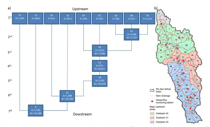
**Figure 3.** a) Calibration order of the Rio das Velhas sub-basins. A: subbasin area (km<sup>2</sup>); AC: accumulated upstream subbasin area (km<sup>2</sup>). b) three major upstream areas, subbasins, and respective water flow stations group.
