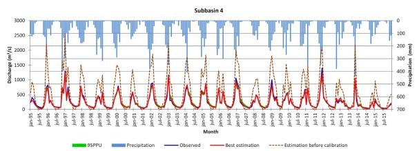
Figure 4. Observed and simulated flows before and after calibration to sub-basin.
