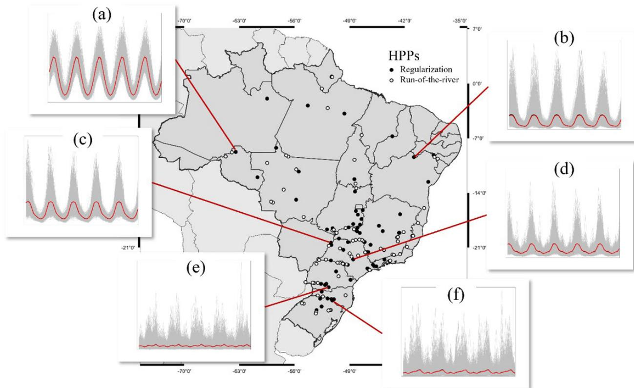
**Figure 3.** HPPs considered in the study, classified according to the type of reservoir. The synthetic flow series shown refer to the plants (a) Samuel, (b) Sobradinho, (c) Ilha Solteira, (d) Barra Bonita, (e) Gov. Bento Munhoz (Foz do Arcaia), (f) Barra Grande. The red lines display historical monthly average flows, the black lines represent synthetic monthly average flows, and the gray lines show the synthetic series.
