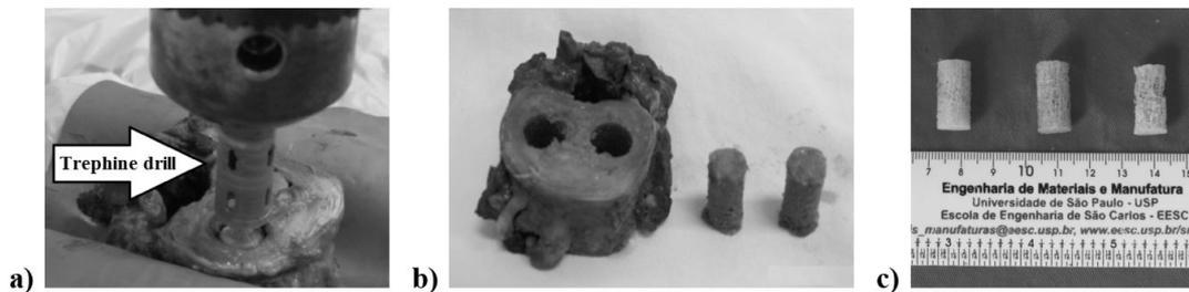
**Figure 1.** (a) Vertebral body trephine drill penetration; (b) Cylindrical specimens of trabecular bone; (c) Specimens (20x10) mm without bone marrow of L<sub>1</sub> region, classified as normal, osteopenic and osteoporotic.
