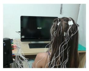
Figure 2. The experimental setup used for the VEP experiments. The volunteers sat comfortably in a chair while a set of images were presented on a computer screen placed at a distance of 70 cm. EEG data were collected throughout the experiment along with a synchronization signal used to indicate the presentation and valence of each image.
