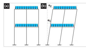
Figure 2 - Structure without (a) or with (b) global geometric imperfections.
