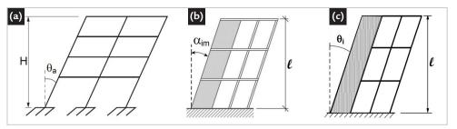
Figure 3 – Out-of-plumb columns in NBR 6118:2014 (a), Model Code 2010 (b) and Eurocode 2 (c) (adapted from ABNT, 2014; FIB, 2010; and CEN, 2004).
