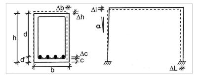
Figure 1 - Different types of deviations (adapted from Zilch and Schießl, 2010).
