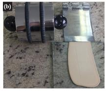
Figure 2 - Images of the no-pick-up time test for samples (a) without lignin and (b) containing 1.00 wt. %.
