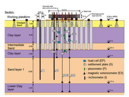
Figure 3 - Soil profile adopted after the installation of the working platform and stone columns with the instrumentation positions (Almeida *et al.*, 2014).
