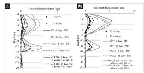
Figure 7 - Horizontal displacement profile - inclinometer 1(a) and 2(b) - Mohr Coulomb (MC) and Cam-Clay (CC) analysis.
