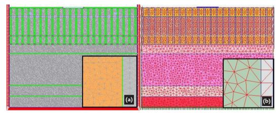
Figure 4 - Mesh used for the model in RS<sup>2</sup> (a) and Plaxis 2D (b).
