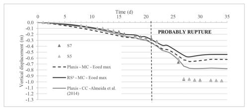
Figure 6 - Vertical displacements - Mohr Coulomb (MC) and Cam-Clay (CC) analysis.
