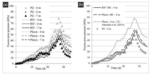
Figure 8 - Excess pore pressure over time in different depths (a) and compared with Cam-Clay (CC) analysis (b).
