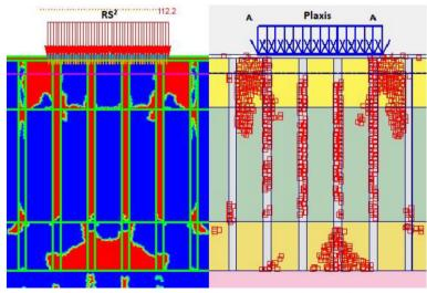
Figure 9 - Yielding points model at Plaxis and RS<sup>2</sup> software.
