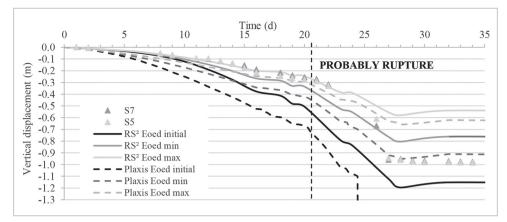
Figure 5 - Vertical displacements comparison.
