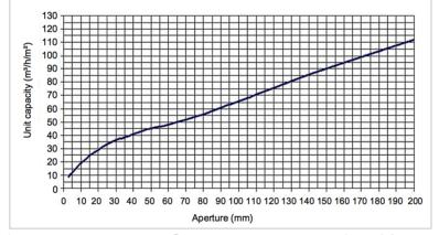
Figure 1 - Volumetric unit capacity –  $Q_{u}^{F}$  versus Screen aperture (Adapted from Metso, 2008).
